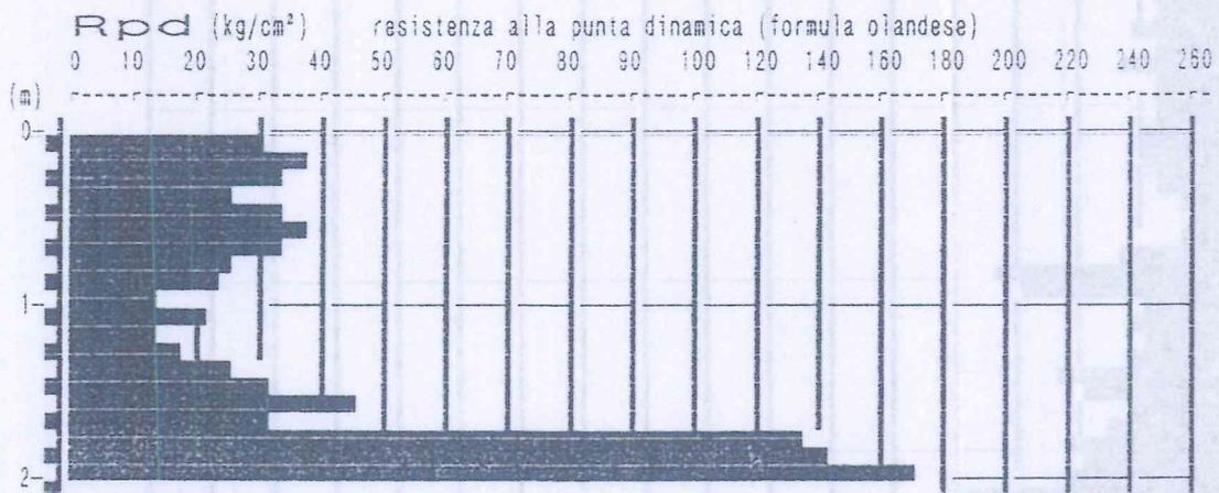
PROVA PENETROMETR. DINAMICA DL 6
